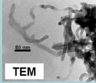
Fig. 1: carbon nanotubes
